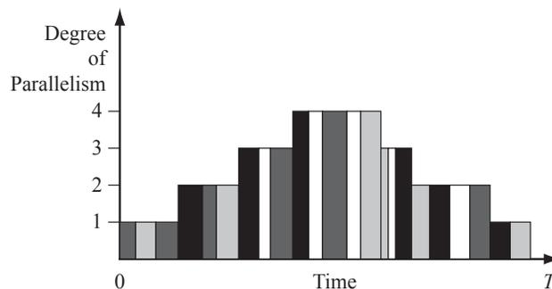
Fig. 1. Parallelism profile of an application.
