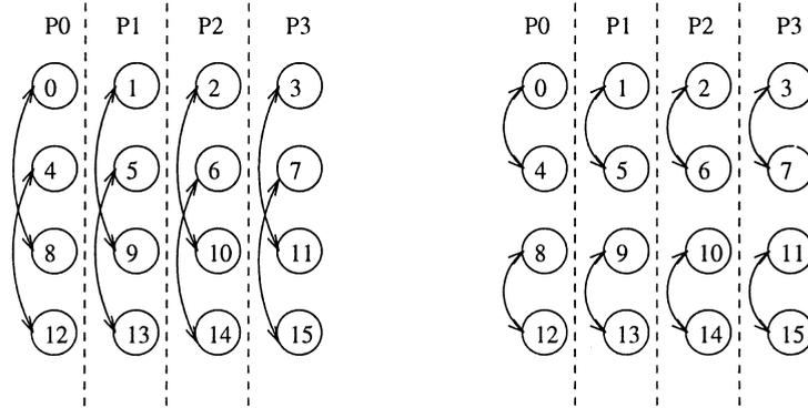
(a). Steps in Phase 1 of the transpose (before transpose)
