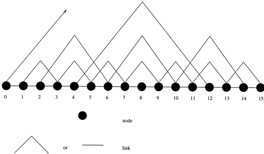
Fig. 1. A 16-node 1-D PEC network.
