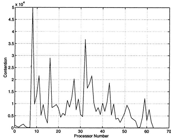
Fig. 18. 2-D mesh contention on each processor (64 nodes,  $m = 2^{10}$ ) all-to-all broadcast, 64 nodes,  $m = 2^{10}$ .
