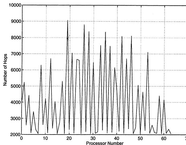
Fig. 13. 2-D PEC network dataflow hops of each processor all-to-all broadcast, 64 nodes,  $m = 2^{10}$ .
