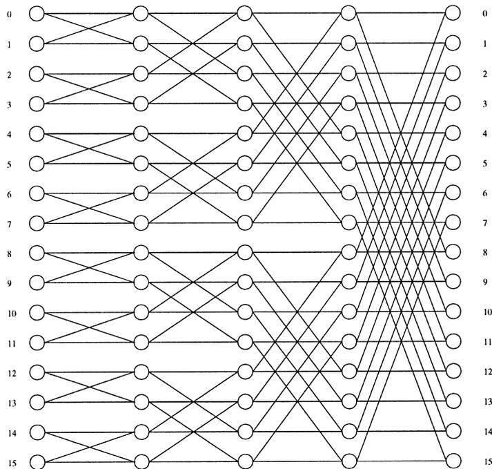
Fig. 10. Binary-exchange scheme.
