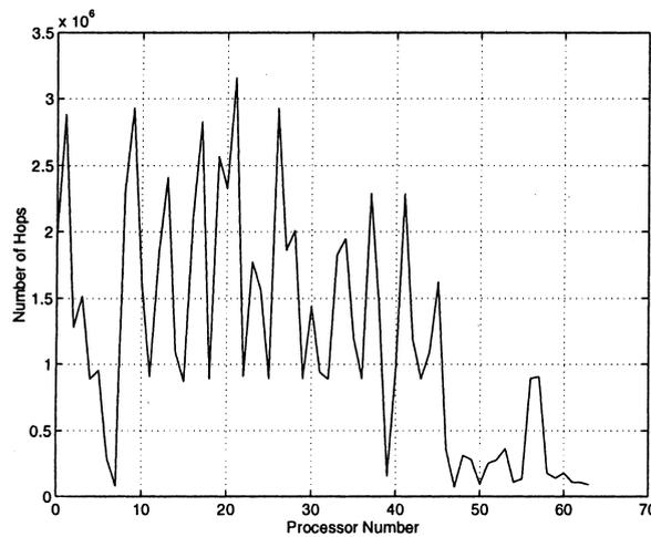
Fig. 21. 2-D PEC network dataflow hops of each processor FFT, 64 nodes,  $m = 2^{18}$ .
