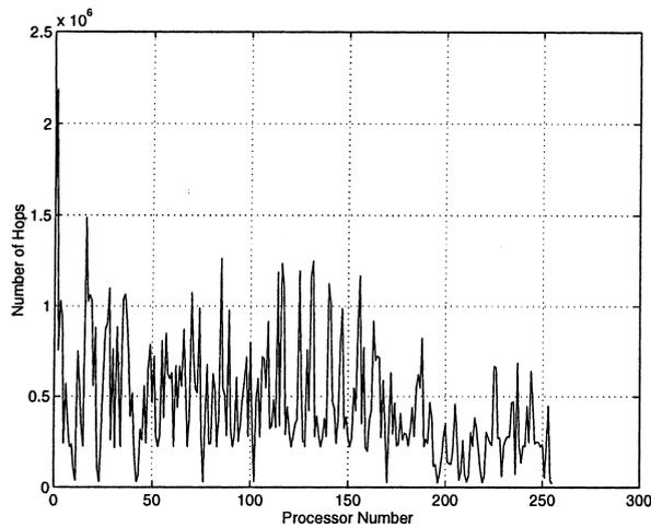
Fig. 23. 2-D PEC network dataflow hops of each processor FFT, 256 nodes,  $m = 2^{18}$ .
