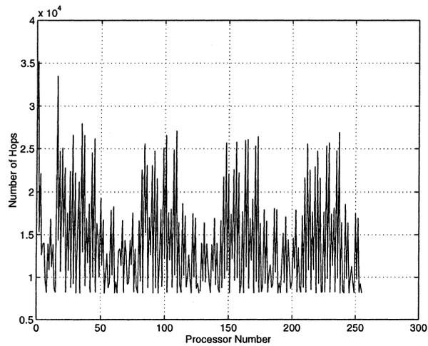
Fig. 15. 2-D PEC network dataflow hops of each processor all-to-all broadcast, 256 nodes,  $m = 2^{14}$ .
