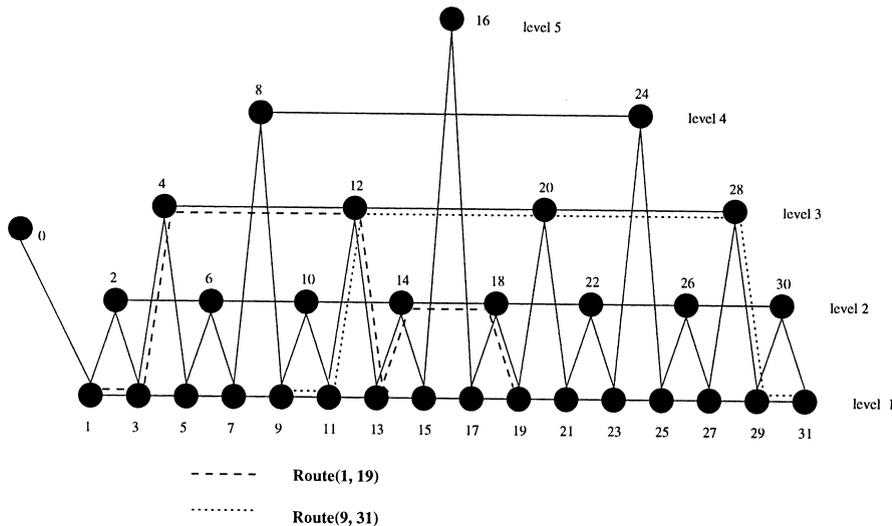
Fig. 5. An *R-Route* path for  $(i, j)$  pair of nodes.
