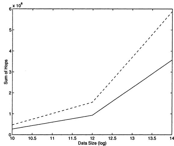
Fig. 27. Comparison of hops. Comparison of all-to-all broadcast with 256 processors.
