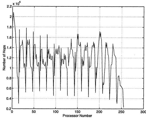
Fig. 24. 2-D mesh dataflow hops of each processor FFT, 256 nodes,  $m = 2^{18}$ .
