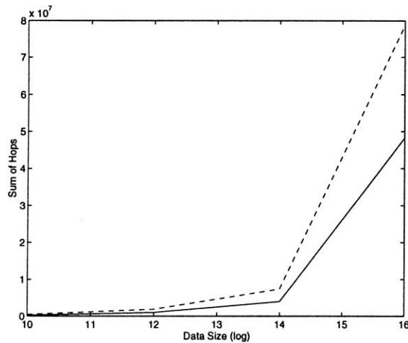
Fig. 25. Comparison of hops. Comparison of all-to-all broadcast with 64 processors.
