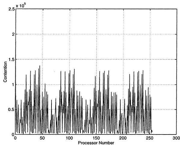
Fig. 19. 2-D PEC network contention on each processor (256 nodes,  $m = 2^{14}$ ) all-to-all broadcast, 256 nodes,  $m = 2^{14}$ .
