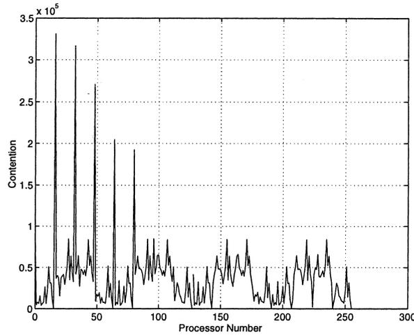
Fig. 20. 2-D mesh contention on each processor (256 nodes,  $m = 2^{14}$ ) all-to-all broadcast, 256 nodes,  $m = 2^{14}$ .
