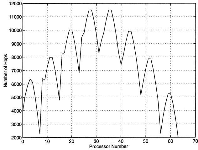
Fig. 14. 2-D mesh dataflow hops of each processor all-to-all broadcast, 64 nodes,  $m = 2^{10}$ .
