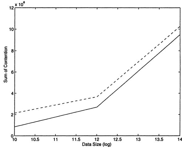
Fig. 28. Comparison of contention. Comparison of all-to-all broadcast with 256 processors.
