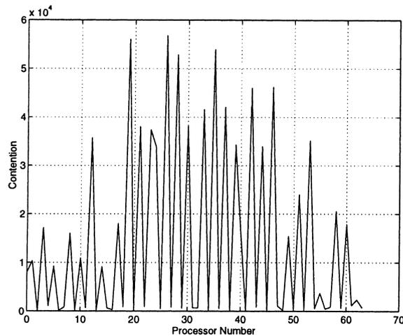
Fig. 17. 2-D PEC network contention on each processor (64 nodes,  $m = 2^{10}$ ) all-to-all broadcast, 64 nodes,  $m = 2^{10}$ .
