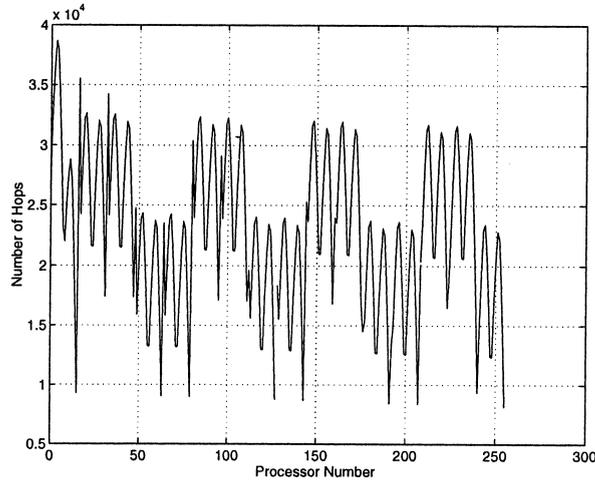
Fig. 16. 2-D mesh dataflow hops of each processor all-to-all broadcast, 256 nodes,  $m = 2^{14}$ .
