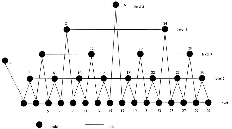
Fig. 2. An alternative representation of a 32-node PEC network.
