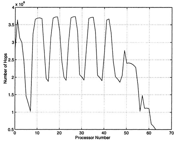
Fig. 22. 2-D mesh dataflow hops of each processor FFT, 64 nodes,  $m = 2^{18}$ .
