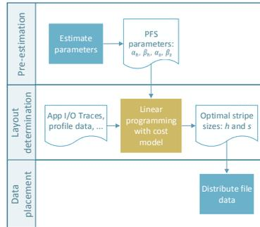
**Fig. 3.** The procedure of the performance-aware data placement scheme
