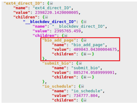
Fig. 1. Function graph of 100MB write() to SSD where value is in \mu s
