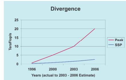
**Figure 1. “Divergence Problem” - Increasing gap between peak performance and sustained system performance (SSP)**
