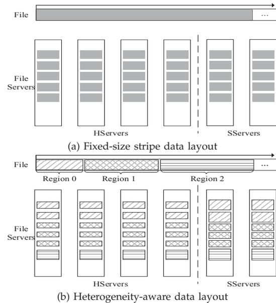
**Fig. 2: Two data layout schemes in a hybrid parallel file system.** This figure shows how a file’s data are distributed on HServers and SServers, focusing on the stripe size configuration. The height of the rectangle on each server represents the stripe size assigned to them. While case (a) uses a fixed-size stripe for each server within the whole file, case (b) divides a file into multiple regions and uses varied-size stripes for HServers and SServers to distribute data in each region.
