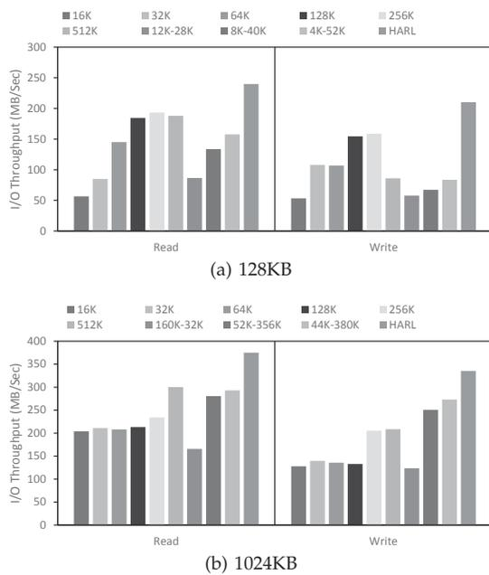
Fig. 10: Throughputs of IOR with various request sizes
