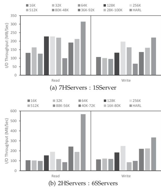
Fig. 11: Throughputs of IOR with various server configurations
