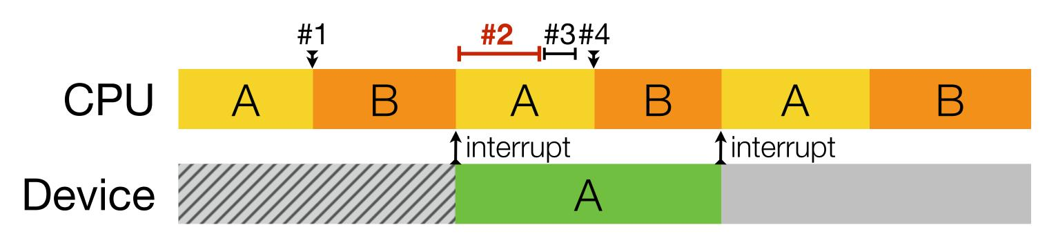
May be able to have device copy data from RAM directly (CPU just provides address as part of command)
