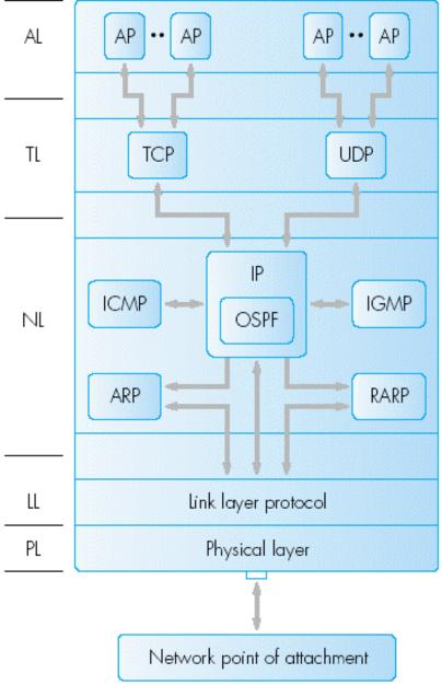
AP = application protocol/process IP = Internet protocol ARP = address resolution protocol RARP = reverse ARP ICMP = Internet control message protocol IGMP = Internet group message protocol OSPF = open shortest path first
